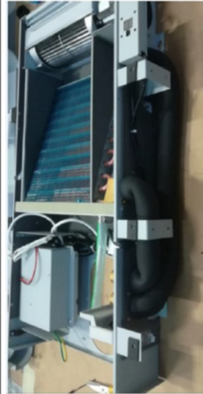
PUT INSULATION IN ALL THE EXTERNAL PIPE
